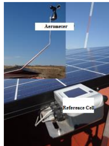
Figure 1 Reference cell and anemometer used to measure wind speed and irradiance respectively.
